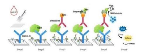
Step1: Wash plate 2 times before adding Standard, Sample (diluted at least 1/2 with Sample Dilution Buffer) and Control (blank) wells!
